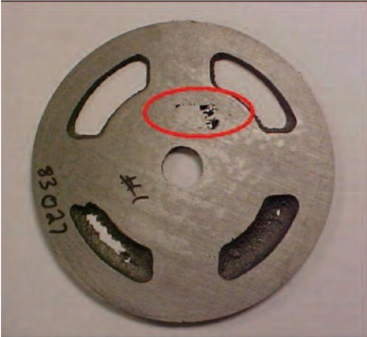
Figure 2. Slice through the left casting, showing shrinkage.
